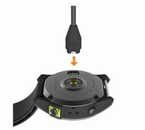
2 Plug the other end of the cable into a USB charging port. The watch displays the current battery charge level.
